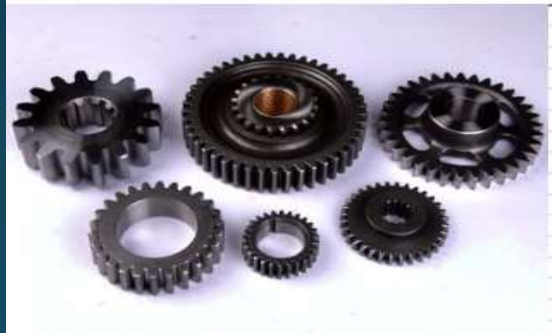
SPUR GEARS- HOBBED, SHAVED AND GROUND
